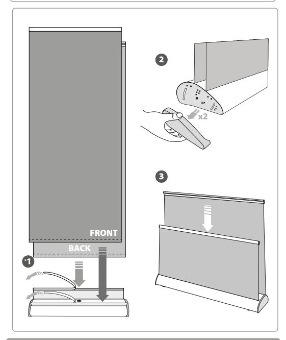
3. SET UP THE ROLL UP **STRUCTURE**
